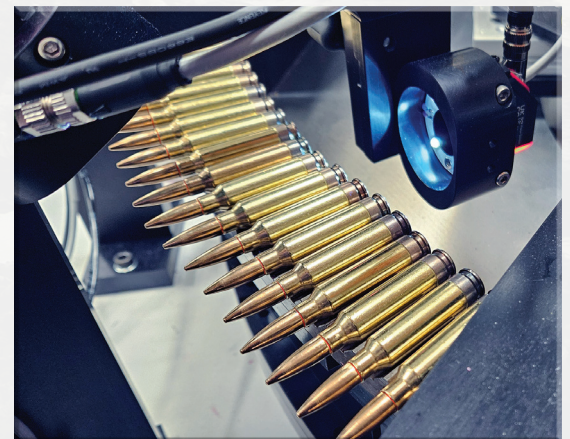
Inside View Of The Autosealer® 5550 Primer Vision Inspection
